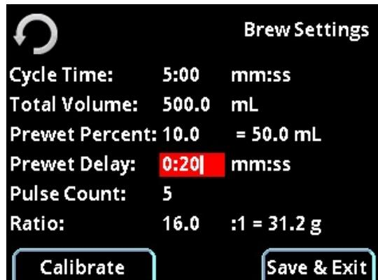
10. The water can be dispensed in a series of pulses. The number of pulses can be set by touching the number next to **Pulse Count**. Rotate the encoder to increase or decrease in 1 pulse increments, push the joystick up or down to change in 1 pulse increments and left or right to change in 10 pulse increments. Press the centre of the joystick to set. (minimum 1, maximum 12 pulses).
