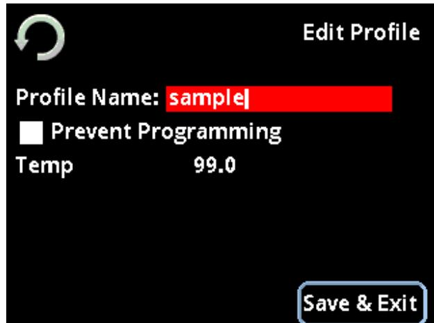
3. Set the heat zone temperatures if desired. To change the set temperature, simply touch the temperature value on the screen and the value will be highlighted. Rotate the encoder left or right to change the value in 1-degree increments. Press the joystick up or down to change the temperature in 1/10 degree increments. Press the center button on the joystick to save the change.
