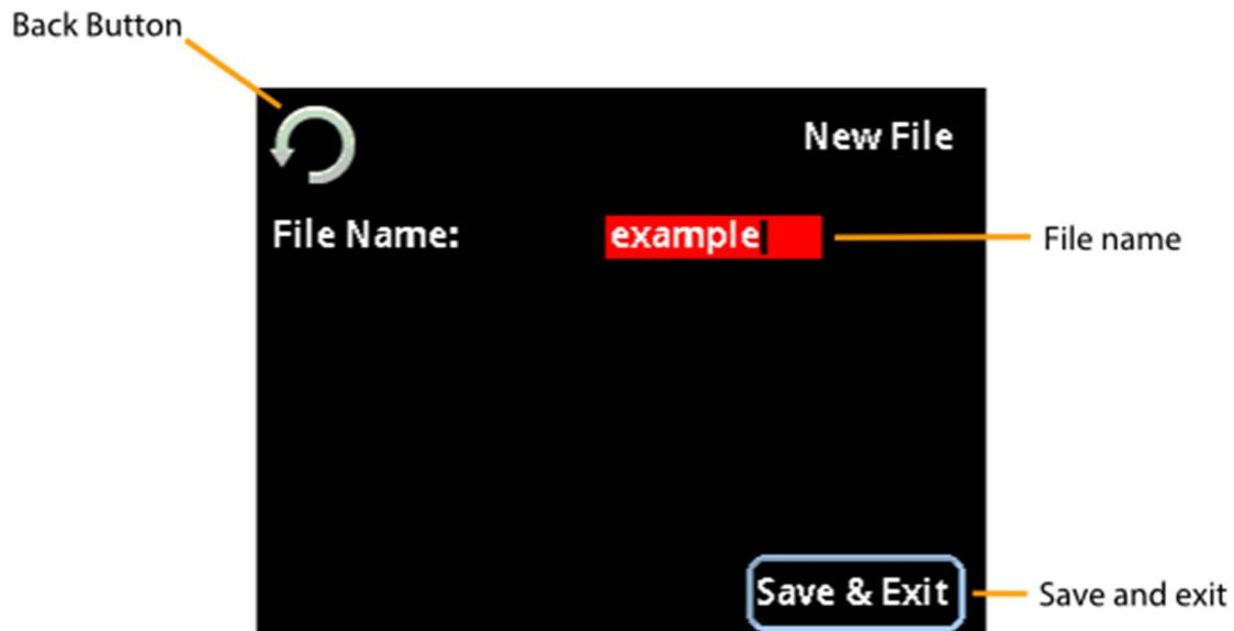
**File name:** This is a descriptive name for the settings file. Touch the name to highlight the field, use the encoder wheel and push-button to rename the file if desired.
